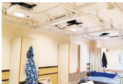
晚間智能監察系統 eNightLog Smart Bed-leaving Monitoring System
